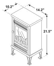
Figure 1 - Heater Dimensions
